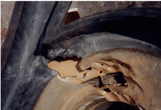
Figure 9: Wear caused by high silica content (wear on rubber lining from centrifugal pump in wet limestone system)
